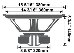
**Woofer Cut Out Diameter:** 16 15/16" (430mm) **Woofer Mounting Depth:** 7 11/16" (195mm)
