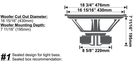
Sealed design for tight bass. Sealed box recommendation: 1.75-2.25cu.ft.
